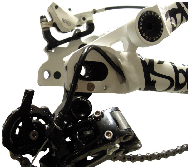
Fig. 22 Internal cable routing for rear derailleur
