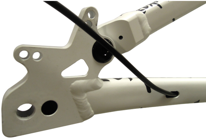
Fig. 23 Internal cable routing for rear disk brake
