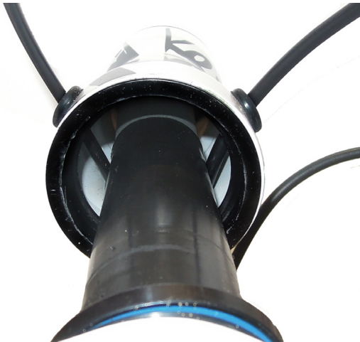
Fig 20. Internal cable routing inside headtube. Steertube protector
