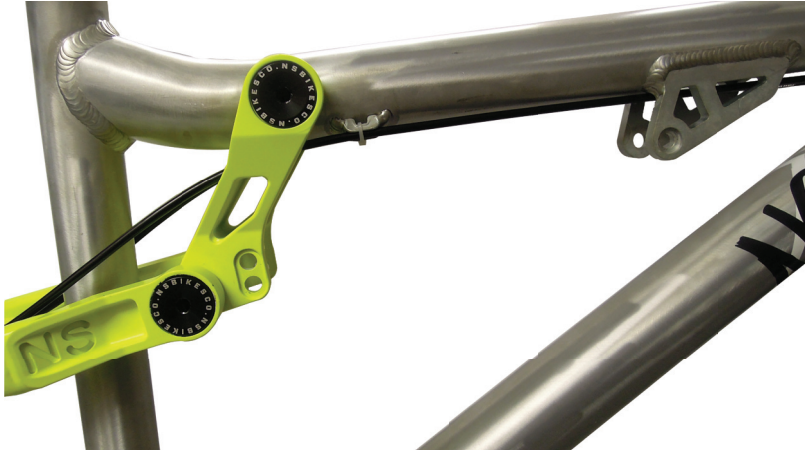
Fig 16. Soda / Soda Slope external cable routing
