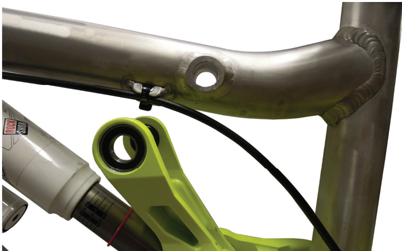
Fig 17. Rocker arm disassembled from top tube (hydraulic brakes)
