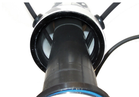
Fig 3. Internal cable routing inside the headtube. Steertube protector.
