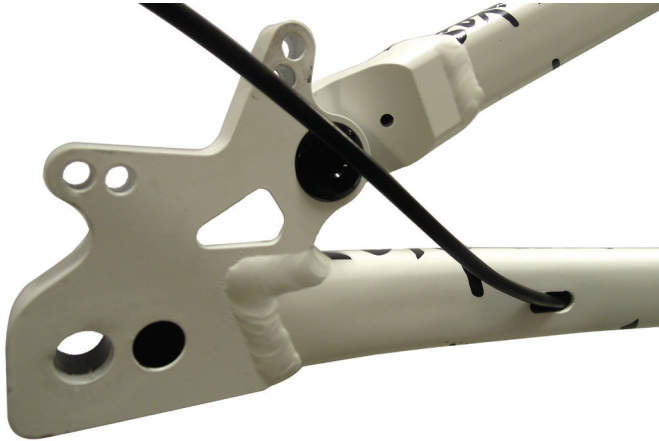
Fig. 23 Internal cable routing for rear disk brake
