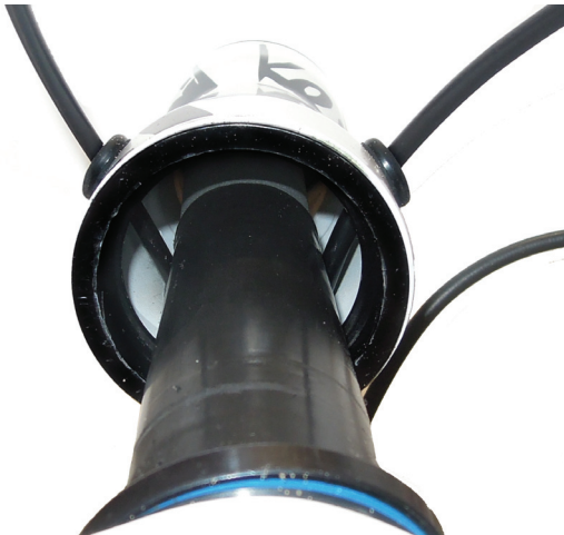
Fig 20. Internal cable routing inside headtube. Steertube protector
