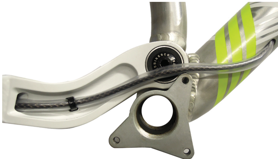
Fig. 21. Internal cable routing in DT/ BB / CS yoke area. Cable housing protector.
