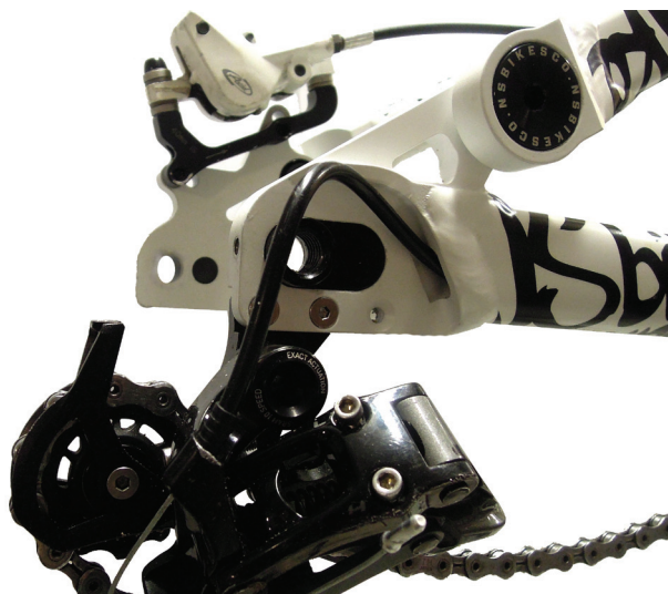
Fig. 22 Internal cable routing for rear derailleur
