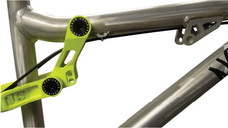
Fig 16. Soda / Soda Slope external cable routing
