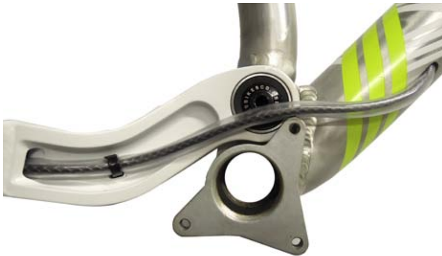
Fig. 18. Internal cable routing in DT/BB / CS yoke area. Cable housing protector.
