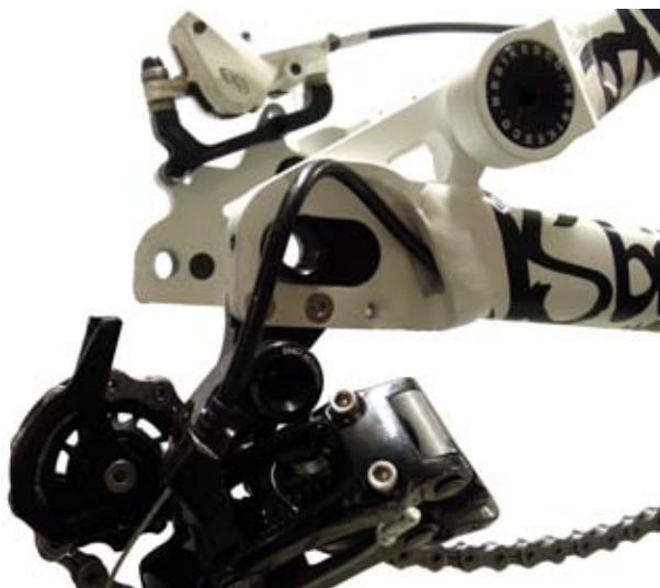
Fig. 19 Internal cable routing for rear derailleurs
