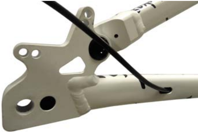
Fig. 20 Internal cable routing for rear disk brake
