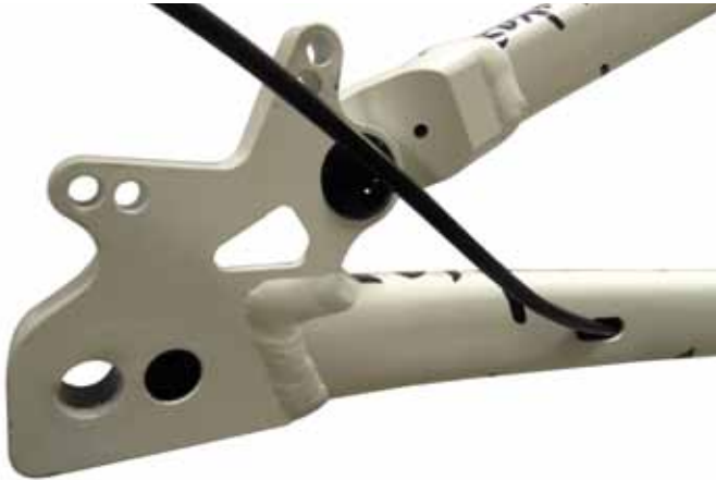
Fig. 23 Internal cable routing for rear disk brake
