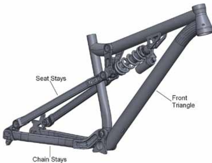
Fig. 1 Soda EVO frame main parts
