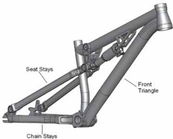
Fig. 5 Soda Slope frame main parts
