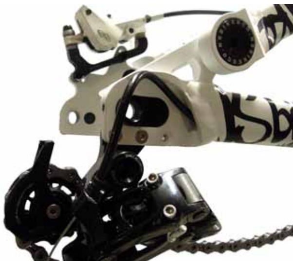
Fig. 22 Internal cable routing for rear derailleur
