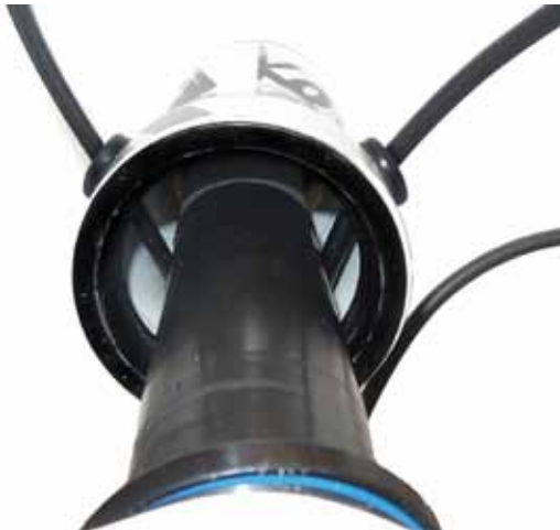
Fig 20. Internal cable routing inside headtube. Steertube protector
