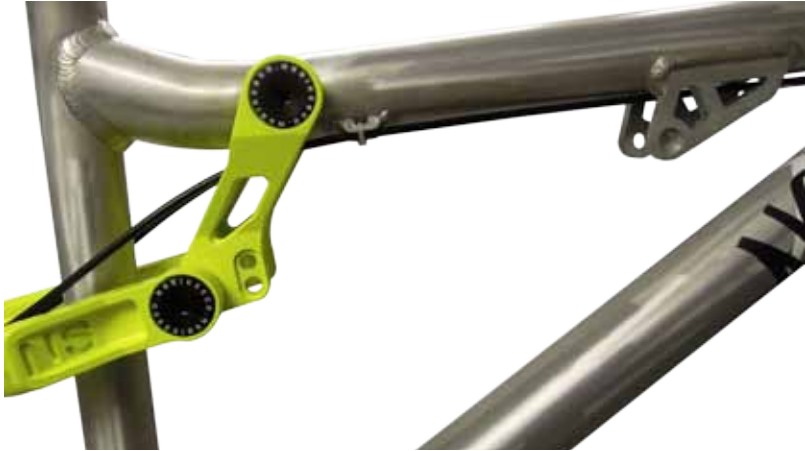
Fig 16. Soda EVO / Soda Slope external cable routing
