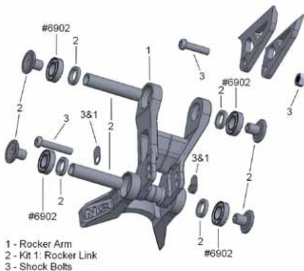
Fig. 2 Soda EVO frame rocker arm links details
