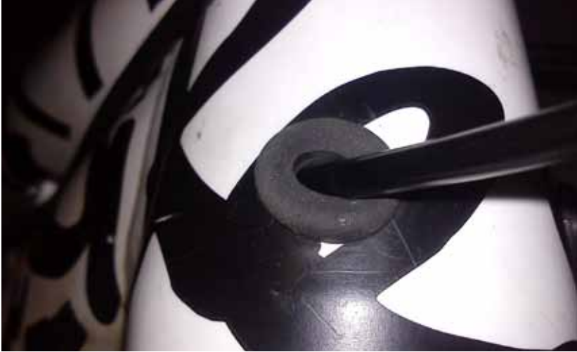
Fig 19 Headtube rubber grommet protector
