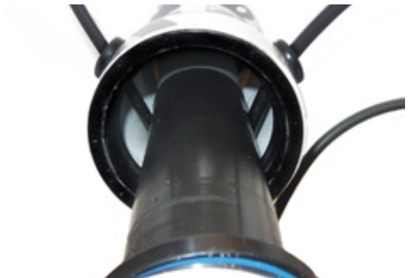
Fig 3. Internal cable routing inside the headtube. Steertube protector.
