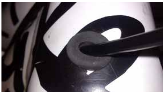
Fig. 2 Headtube rubber grommet protector
