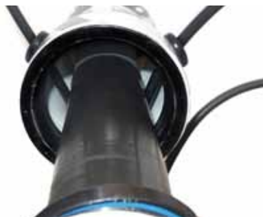
Fig 3. Internal cable routing inside the headtube. Steertube protector.
